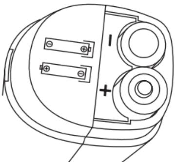
3. Place the cover back onto the battery compartment until you feel it click into place.
